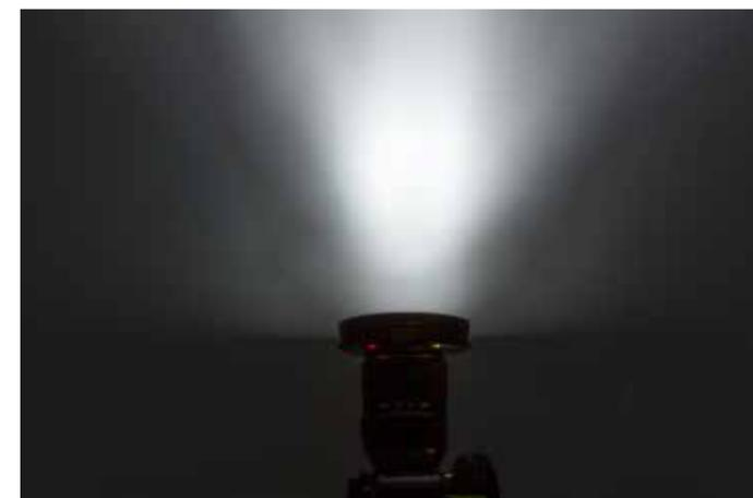
Fig. 2: Light distribution from the Ring Flash Metz MS-1
