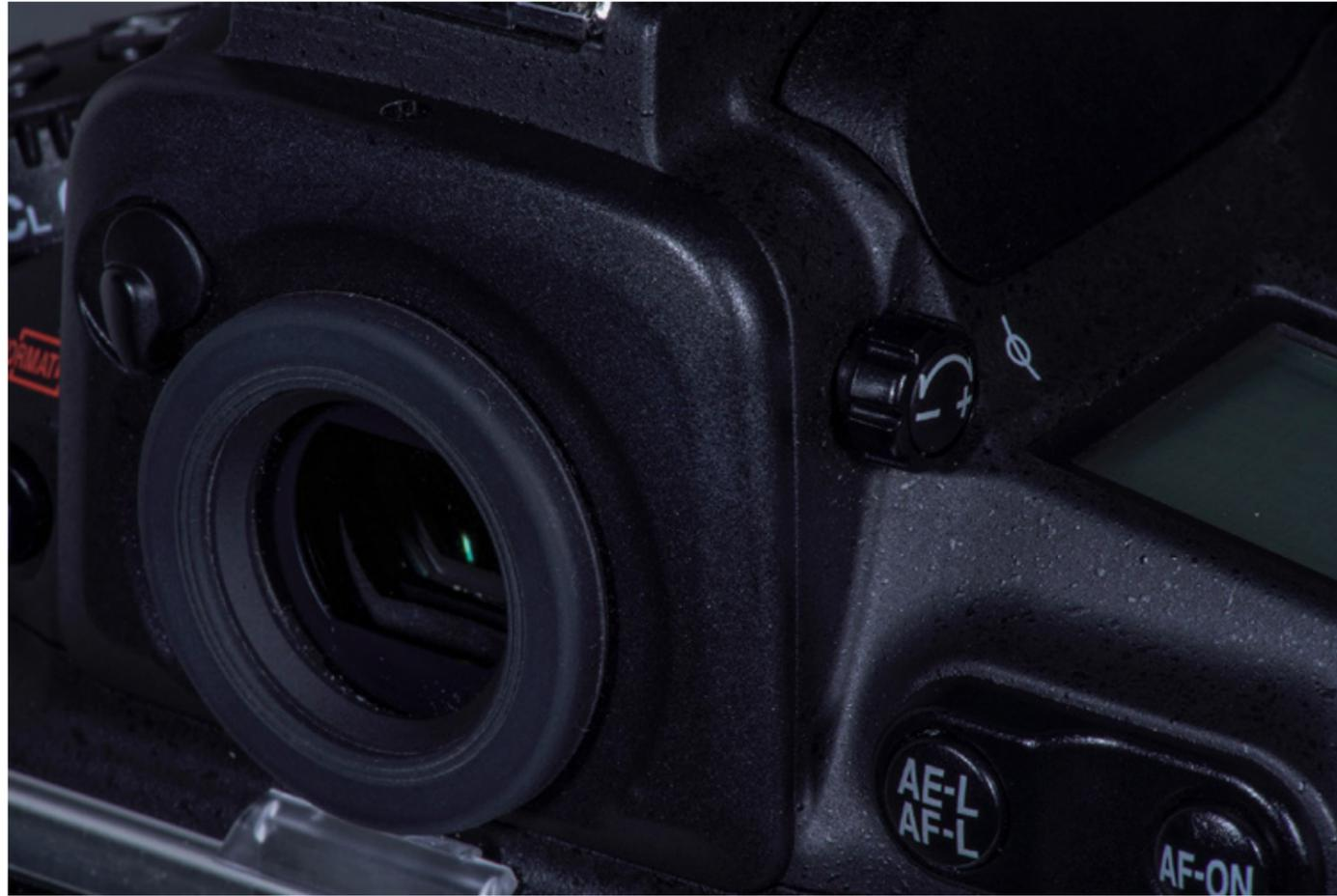
Fig. 2: Diopter adjustment wheel on a Nikon DSLR
