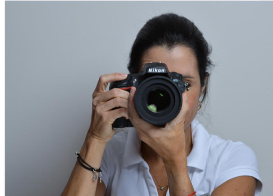
Fig. 3: The correct hold of the camera using right and left hand
